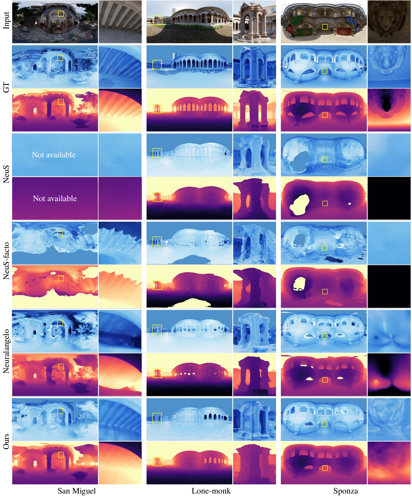
Figure 5. We compare our method with traditional and neural methods using ground-truth geometry. We present qualitative results of NeuS [28], NeuS-facto [33] and Neuralangelo [15] here; our method produce higher-quality 3D geometry. Please refer to Table 2 for complementary quantitative evaluation and to supplemental material for further qualitative comparisons of omitted traditional methods, including COLMAP [21], and Ego-centricRecon [8].
